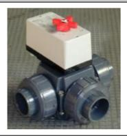
For smaller installations with up to 24 panels (3 banks), flow diversion through the solar panels is normally achieved by installing a Suncell 3-Port Motorised Valve in the filtration circuit after the filter, to divert water to the panels when the Solax controller switches to heating mode.
